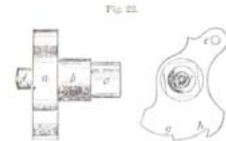
Fig. 22. Tumbler, full size. a , body; b , arbor; c , square; d , pivot; e , swivel-arm and pin-hole; f , tumbler-screw hole; g , cock-notch; h , half-cock notch.
