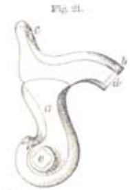
Fig. 21. Hammer, half size. a , body; b , head; c , comb; d , countersink; e , tumbler-hole.
