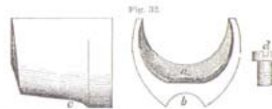
Fig. 32. Tip, full size, (malleable iron.) a , recess for stock; b , groove for ramrod; c , screw-hole; d , screw.
