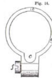
Fig. 15. Bayonet, quarter size. a, blade; b, neck; c, socket; d, bridge; e, stud-mortise; f, clasp.
