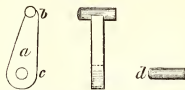
Fig. 20. Mainspring-swivel , full size. a , body; b , axis; c , tumbler-pin hole; d , tumbler-pin.
