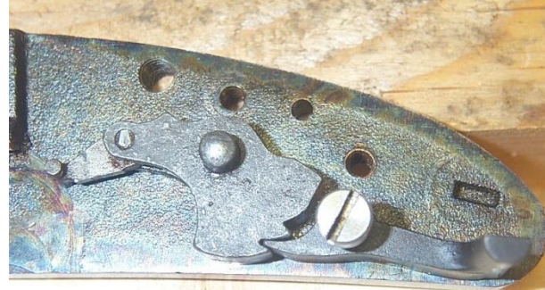
Sear engaged in half cock notch
