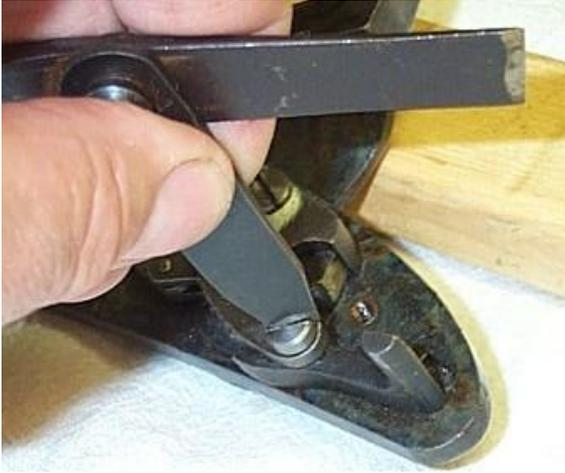
**Step #7** – Install the sear spring and screw. This is pretty much just the reverse of how you removed it. Insert the screw into the loop on the spring and with the spring up out of the way, thread the screw into the lock plate. Stop just a little before it is tight.
