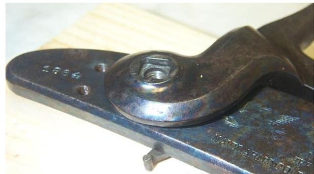
At this point it's a good idea to have a friend hold the lock plate in place while you tap the hammer down on the tumbler. Use a wooden dowel or block of wood and tap it down firmly onto the tumbler.
