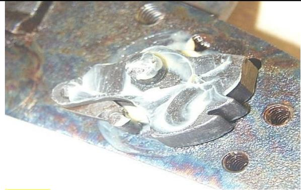
**Step #5** – Press the bridge into place over the tumbler. Be sure the alignment pin goes in the correct hole. Install the bridge screw. Again, check to make sure the tumbler/hammer rotate smoothly.
