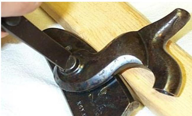
**Step #4** – Put a little lithium grease on the exposed side of the tumbler.
