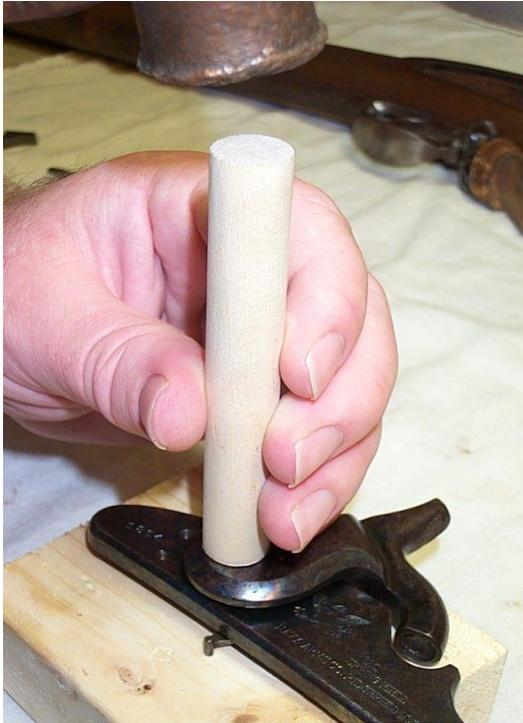
The hammer should go down almost flush with the top of the threaded hole. There needs to be a little clearance between the hammer and lock plate, so the hammer/tumbler set rotates freely on the lock plate. Now install the hammer screw. The screw should not be used to pull the hammer down further onto the tumbler. It is simply there to keep the hammer from coming off the tumbler. Attempting to pull the hammer down with the screw could cause the screw to break off. Not a good thing.
