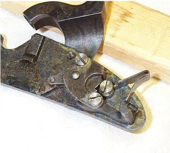
Press the spring down into place against the top of the sear, slightly compressing the spring as it bears against it. Ensure the little tab on back of the spring slips into its slot, then while holding the spring in place, finish tightening the screw.
