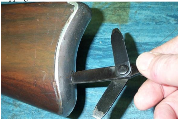
The blade with a convex end is for the butt plate screws.
